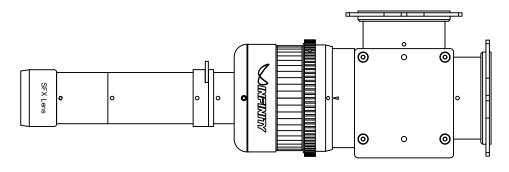
A Dual-port InfiniProbe shown with a Beamsplitter Cube.
