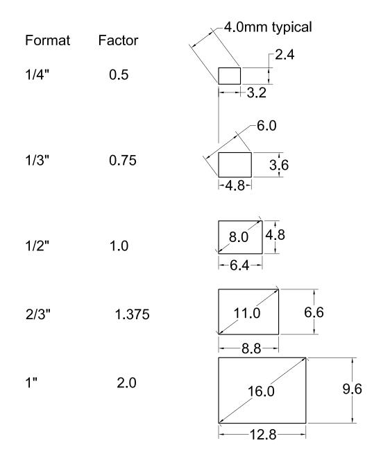
Unless otherwise noted all data is given for 1/2" camera sensors. For FOV or magnification in other sensor sizes use the factors listed. For example, a FOV of 25mm listed for a 1/3" camera would be  $25 \times 0.75 = 18.75$ mm.
